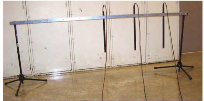
Fig. 3 - Experimental test set-up showing microphones and rack mount. The microphones in the photo have a fixed horizontal spacing of 40 cm.
