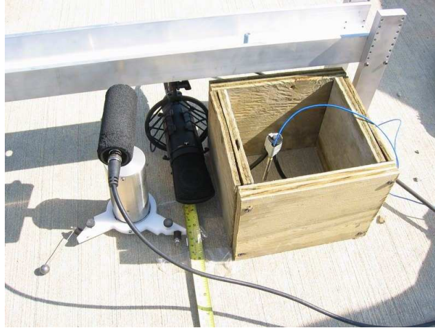
Figure 6.7: The air-coupled MASW testing setup on the CRCP pavement.
