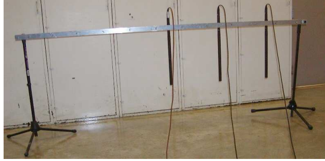
Figure 6.11: Test set-up showing microphones and the rack mount. The microphones in the photo have a fixed horizontal spacing of 40 cm.
