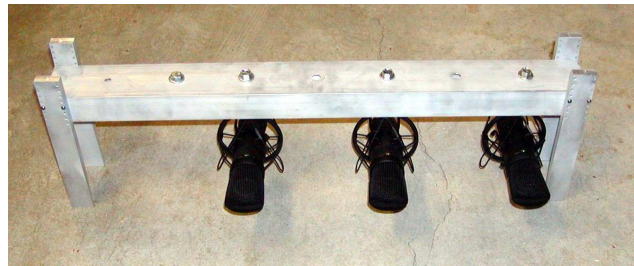
Figure 6.2: Microphone array frame for the air-coupled SASW test.
