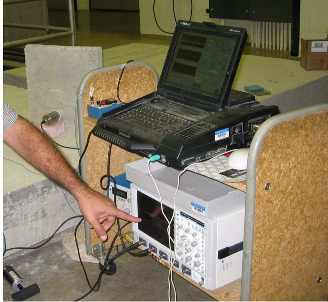
Figure 5.7: Data collecting system. It includes a fieldwork laptop computer and a digital oscilloscope.
